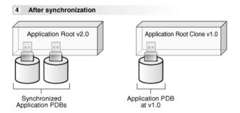
When an application is upgraded, Oracle Database automatically clones the application root.
